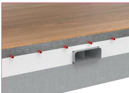
**Under-floor laying:** COMPAIR STEEL flow® is laid under the screed layer, and in case of built-in underfloor heating, directly in the insulation layer. The requirements for noise protection are to be ensured according to the circumstances.
