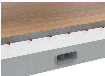
**Concrete laying:** COMPAIR STEEL flow® is cast into the concrete ceiling or concrete floor. The position and arrangement of the ventilation ducts in the concrete are to be checked by the structural engineer.
