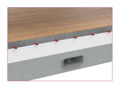
Concrete laying: COMPAIR STEEL flow® is cast into the concrete ceiling or concrete floor. The position and arrangement of the ventilation ducts in the concrete are to checked by the structural engineer.
