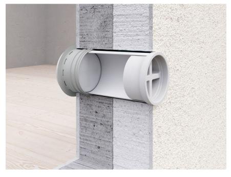
construction set, a core drilling of 162mm - 165mm (standard diameter 150mm) is required. The shell construction set is suitable for all customary wall thicknesses (220mm - 550mm). The flexible wall connection sleeve is hammered into the wall from the kitchen side, together with the wall conduct pipe, and later serves as a direct connection piece for all round duct connections of the duct system.
